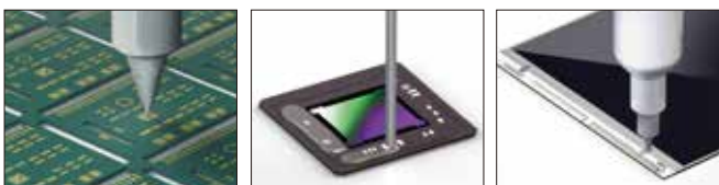
Ag paste dispensing for die bonding
